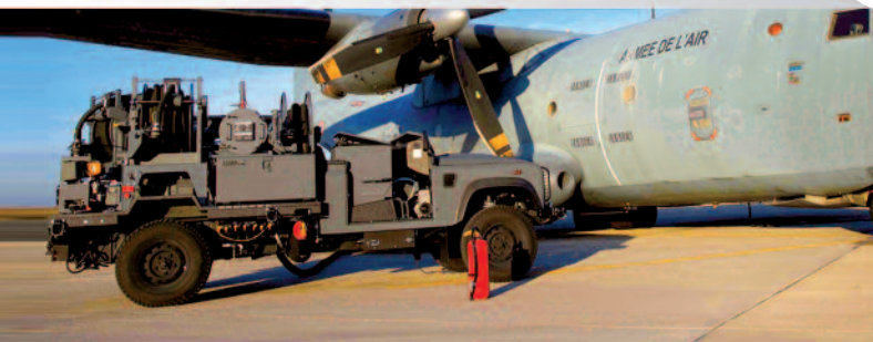
Tactical hydrant dispensers
